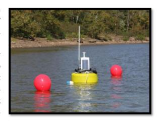
Smart buoys with sensors can also be used to monitor the ecological status of the surrounding waters, detecting any pollutants or harmful substances that may pose a threat to marine life and
