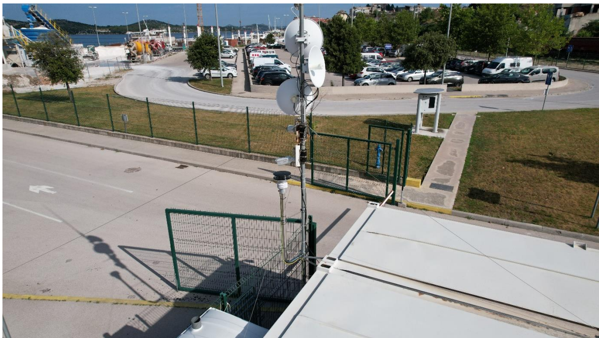
Figure 17. Land sensors for receiving information from buoys 3 (photo made by air drone).
